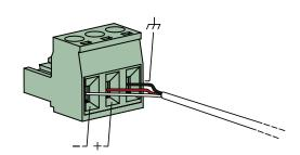
For unbalanced signal input connections
