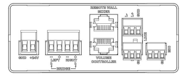
All necessary connections of the AMP22 are provided at the backside of the device. An overview and explanation of all the connectors and possibilities is given below.
