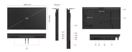
1. Speaker 2. OPS Slot 3. USB 2.0 4. RS-232 5. USB 3.0 6. USB-C 7. HDMI 1(ARC) 8. HDMI 2 9. HDMI OUT 10. HDMI 3 11. Control Panel 12. WiFi Slot 13. VESA® Wall Mount (600x400mm)
