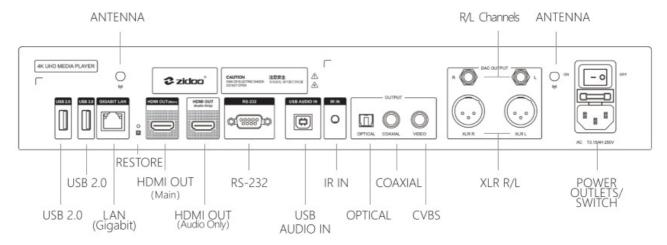
Antennas installation instruction: please install two antennas in the accessories box to the antenna interfaces shown in the diagram above.
