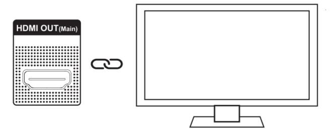
3. Double Output mode (audio and video separate output): please shutdown both TV and Media Player, then connect one HDMI cable from HDMI OUT AUDIO ONLY port to amplifier while connect the other HDMI cable from HDMI OUT MAIN port to TV.
