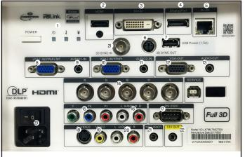
1. Power LED Indicator 9. Audio-In (VGA-1) 2. HDMI 10. VGA 2-In 3. DVI-D 11. Audio-In (VGA-2) 12. VGA-Out
