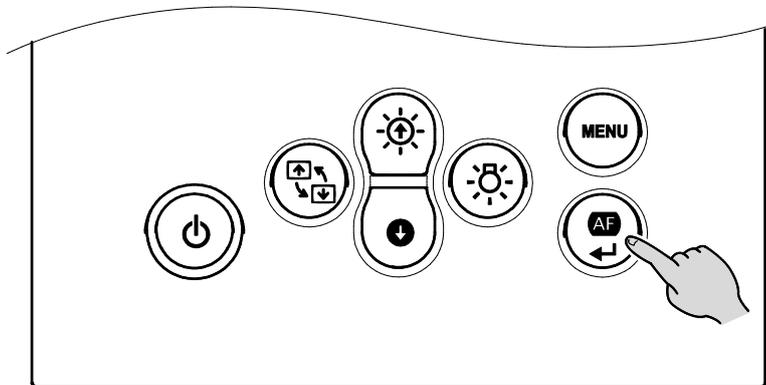
The auto focus can also be performed by pressing the AF button in the camera head.
