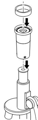
Match the centers of the microscope attachment lens and eyepiece, and use the three screws to evenly tighten the lenses against each other.
