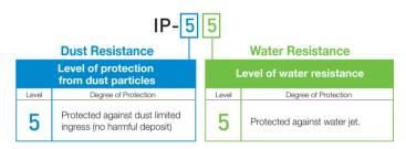
\* What is IP?: This denotes the degree of dust and water resistance. IP is an abbreviation of the international standard Ingress Protection Defined in the IEC60529 international standard.
