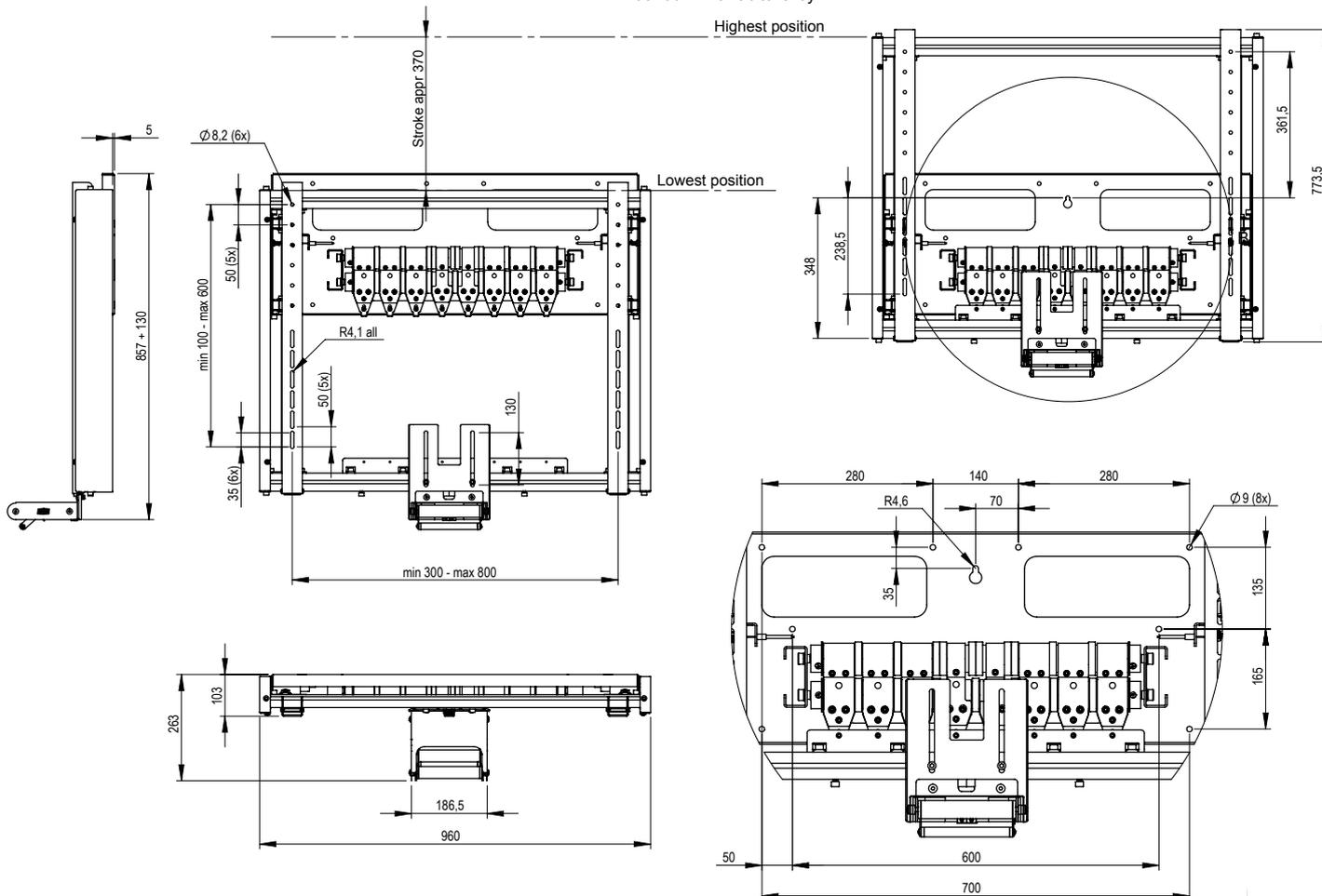
SMS Presence Wall Manual Light technical drawing in mm
