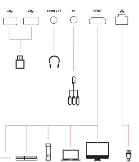
The connectors panel of the JmGO provides connections for external equipment
