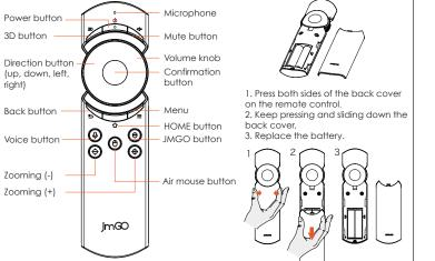
Power button: as JMGO projector is connected to external power supply, gently press the power button to power on:
